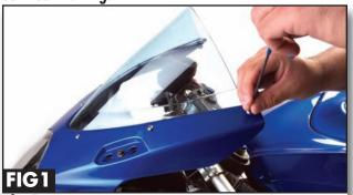
**Fig 1**. Using the appropriate size and type of screw driver or allen head, remove the windscreen screws from the top working your way down and in pairs side to side.
