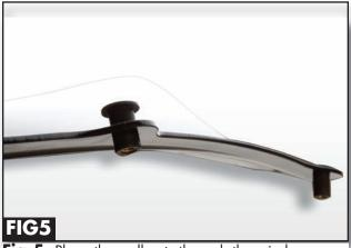
**Fig 5.** Place the well nuts through the windscreen as shown. \*For most modern sportbikes.
