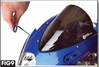
Fig 9. Now tighten the windscreen down with the proper driver starting at the bottom working your way
