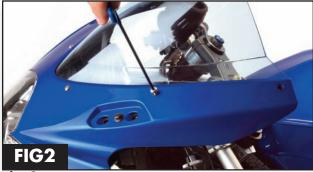
**Fig 2.** As you remove the windscreen screws, check to see if the mirrors attach to the windscreen through the fairing. If they are, you will need to remove them per your repair manual.
