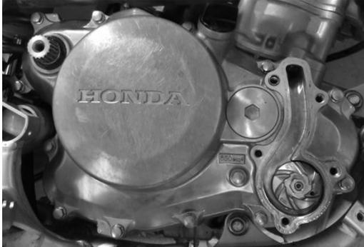
**NOTE:** Be sure that the copper washer for the water pump as well as the sleeve and O-ring for the water jacket are not displaced.
