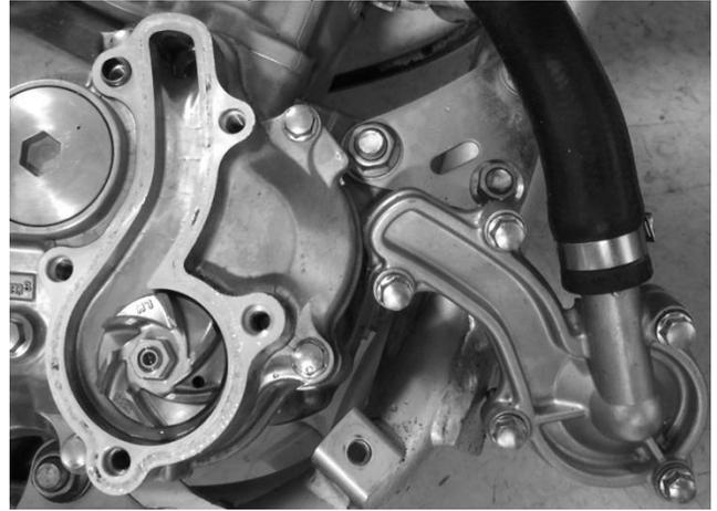
6. Remove the kick starter using a 12mm socket.
