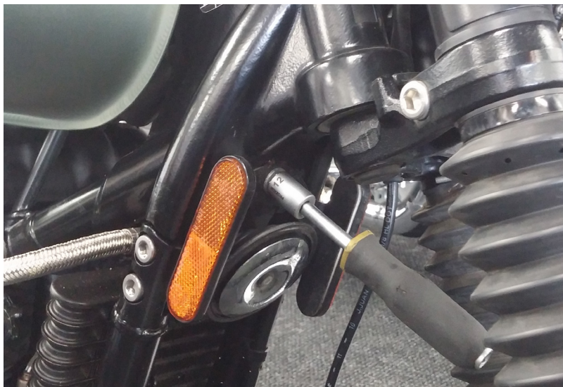
① Use 12mm socket to remove horn.
