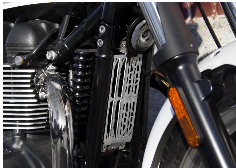
④ Reinstall the horn, make sure horn wires are not pinched.
