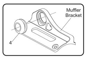
Carefully slide Yoshimura muffler assembly over the stock header outlet. Secure muffler to (1) 13120-BRKT muffler hanger bracket using the hardware provided in the kit.
