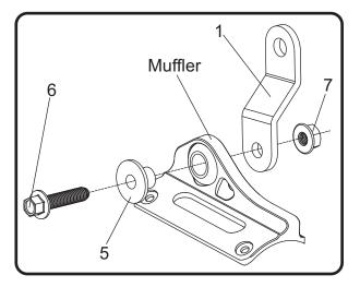
Torque (6) M8X30H muffler mount bolt to 30 Nm (3.0 kg-m, 22 ft-lb).
