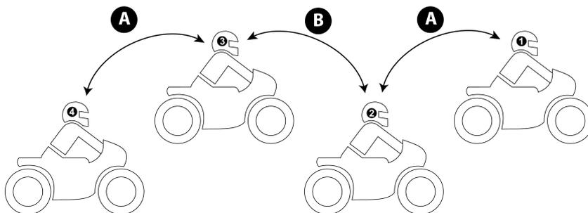
Cardo recommends that during a 3-way or 4-way intercom conference call, a rider that is using mobile phone or GPS navigation should be connected to only one Bluetooth intercom call (riders 1 and 4 in the above diagram) so they can continue to hear mobile phone and GPS announcements.
