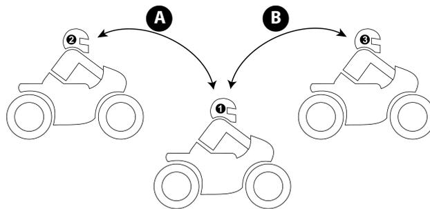
In a 4-way intercom conference call, there are two pairs of riders. In each pair, the riders are connected to each other through channel A. In each pair, one of the riders (riders 2 and 3 in the figure below) is also connected to a rider in the other pair through channel B. All four riders are now all connected in a 4-way Bluetooth intercom call.
