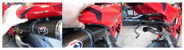
8. Mount the DMP Fender Eliminator using the 6x16 bolts and 6x15 (larger 6mm) washers.
