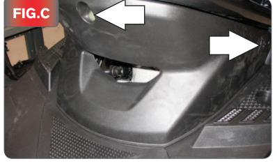
Remove the engine cover by removing the 1 screw in the front and the 2 push tabs (1 on either side) (Fig.C).
