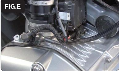
10 Attach the pair of PCFC injector leads with the orange colored wires to the left fuel injector and the stock wiring harness as shown in Figure E.
