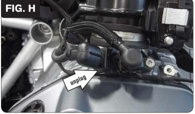
13 Unplug the stock wiring harness from the right fuel injector as shown in Figure H.
