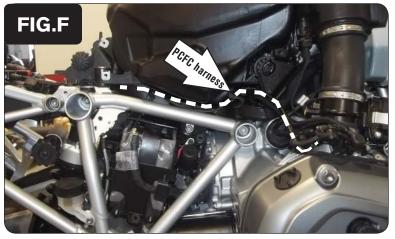
11 Route the PCFC wiring harness branch with the 6mm ring lug and the pair of injector leads with yellow colored wires towards the right engine head following inside the right side frame rail as shown in Figure F.
