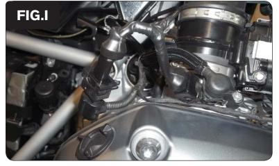
4 Attach the pair of PCFC injector leads with the yellow colored wires to the right fuel injector and the stock wiring harness as shown in Figure I.
