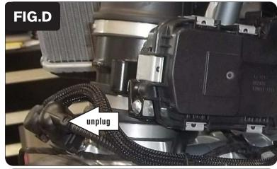
9 Unplug the stock wiring harness from the left fuel injector as shown in Figure D.
