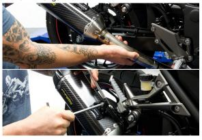
12. Tighten barrel clamp.
