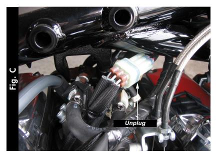
7 Locate the clear 6 pin connector under the main frame spar (Fig. C).
