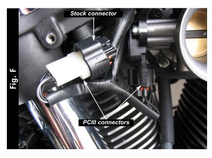
Plug the connectors from the PCIII inline of the stock TPS and stock wiring harness (Fig. F).
